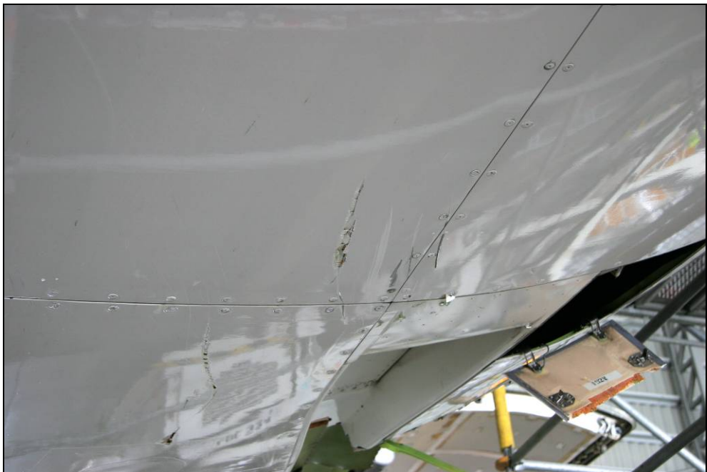
Figure 4. Panel damage to the rear of the rupture site
