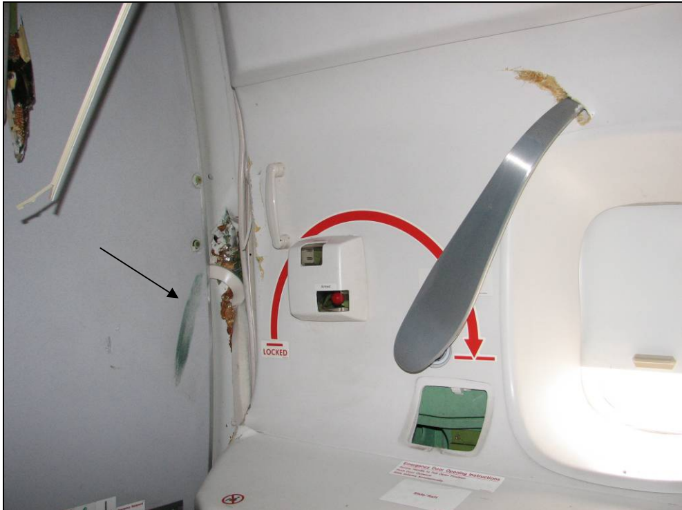
Figure 12: Door frame damage, green paint smear and rotated R2 door handle
