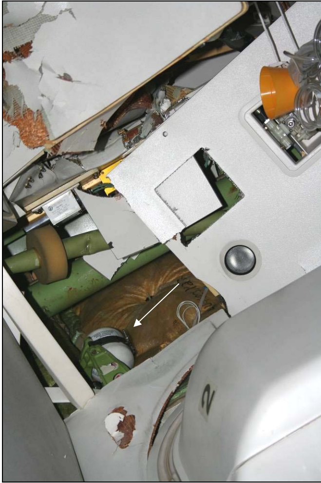
Figure 15: Cut-out section found in panels above the R2 door
