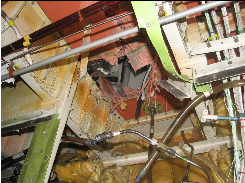
Figure 12: Door frame damage, green paint smear and rotated R2 door handle
