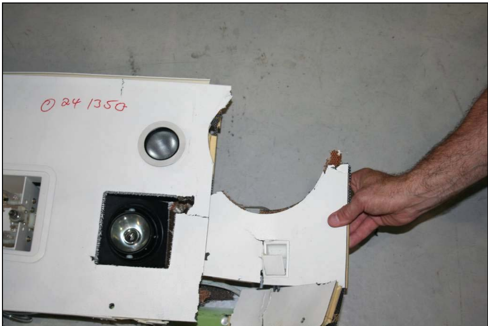
Figure 15: Cut-out section found in panels above the R2 door
