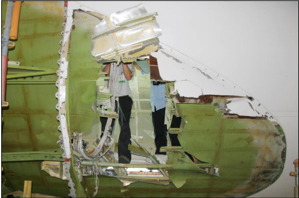
Figure 4. Panel damage to the rear of the rupture site
