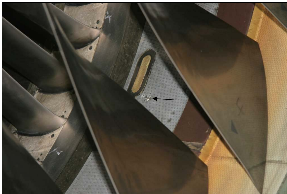
Figure 5: Damage to acoustic lining (arrowed) behind the number-3 engine fan
