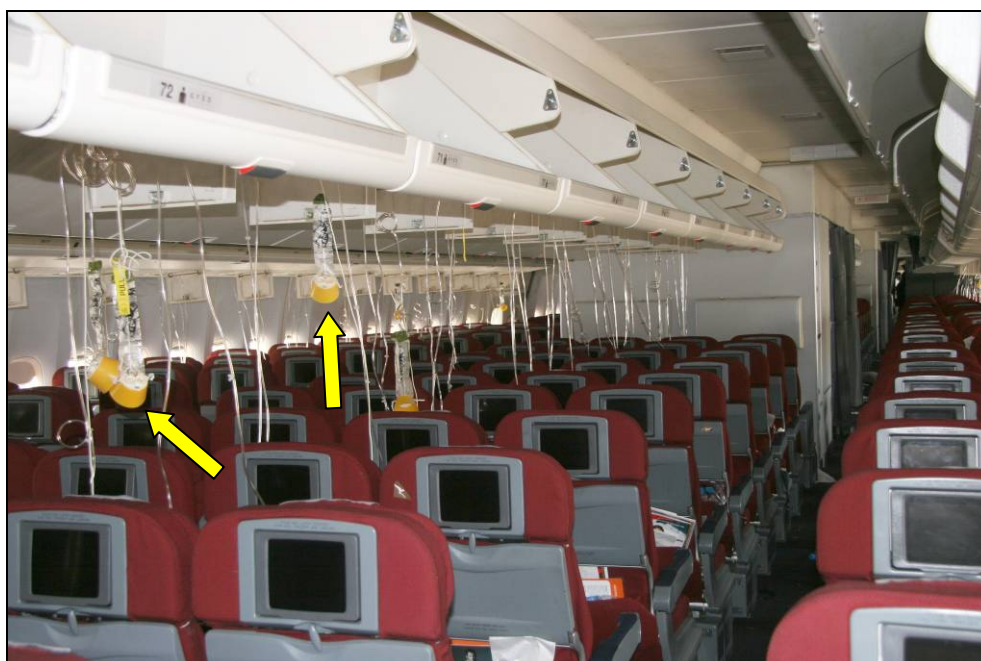
Figure 18: Typical appearance of cabin. Note passenger masks dropped and activated, and those dropped and not activated (arrowed)
